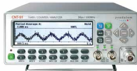
Figure 5: Display showing the trend (signal over time) of sampled data.
