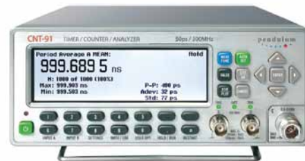
Figure 4: Display showing different statistical parameters viewed at the same time.
